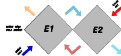
Cross-flow heat recovery plate exchangers can be connected in series to increase the efficiency.
